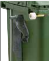
male lifting device fitted on Bologna device
